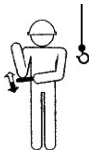
Use Auxiliary Hoist
